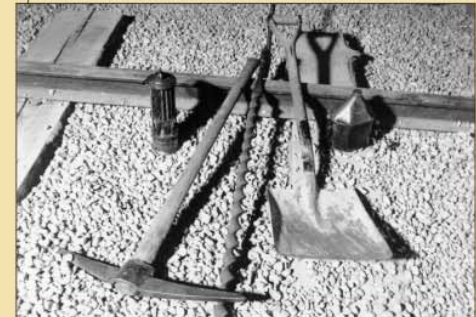
Above are examples of some of the tools required in a mine: A Wolf Safety Lamp, a pick, boring bit, shovel, and copper powder flask for blasting.
